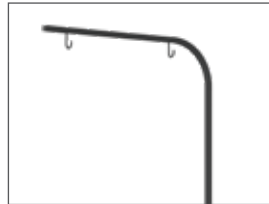
SINGLE 18" arm with 8" on center J hooks.
